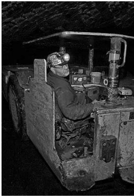
UMWA protections: Shuttle car and enclosed canopy. Earl Dotter, 2006
